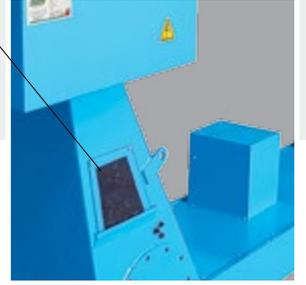
Being different from scraper conveyor, drum filter which can be washed from opposite side, is added to outlet of the cooling liquid. Due to internal washing system, filter cleans itself by washing. Thus, the filter doesn't require maintenance.
