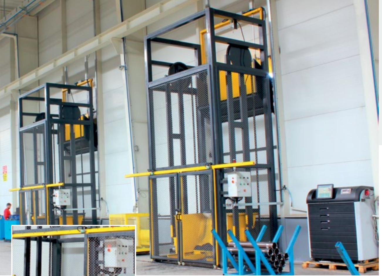
It enables full chip carts to be emptied into container safely. It is manufactured specially according to sizes of container to be loaded. It can carry chip bucket up to 600 kg.
