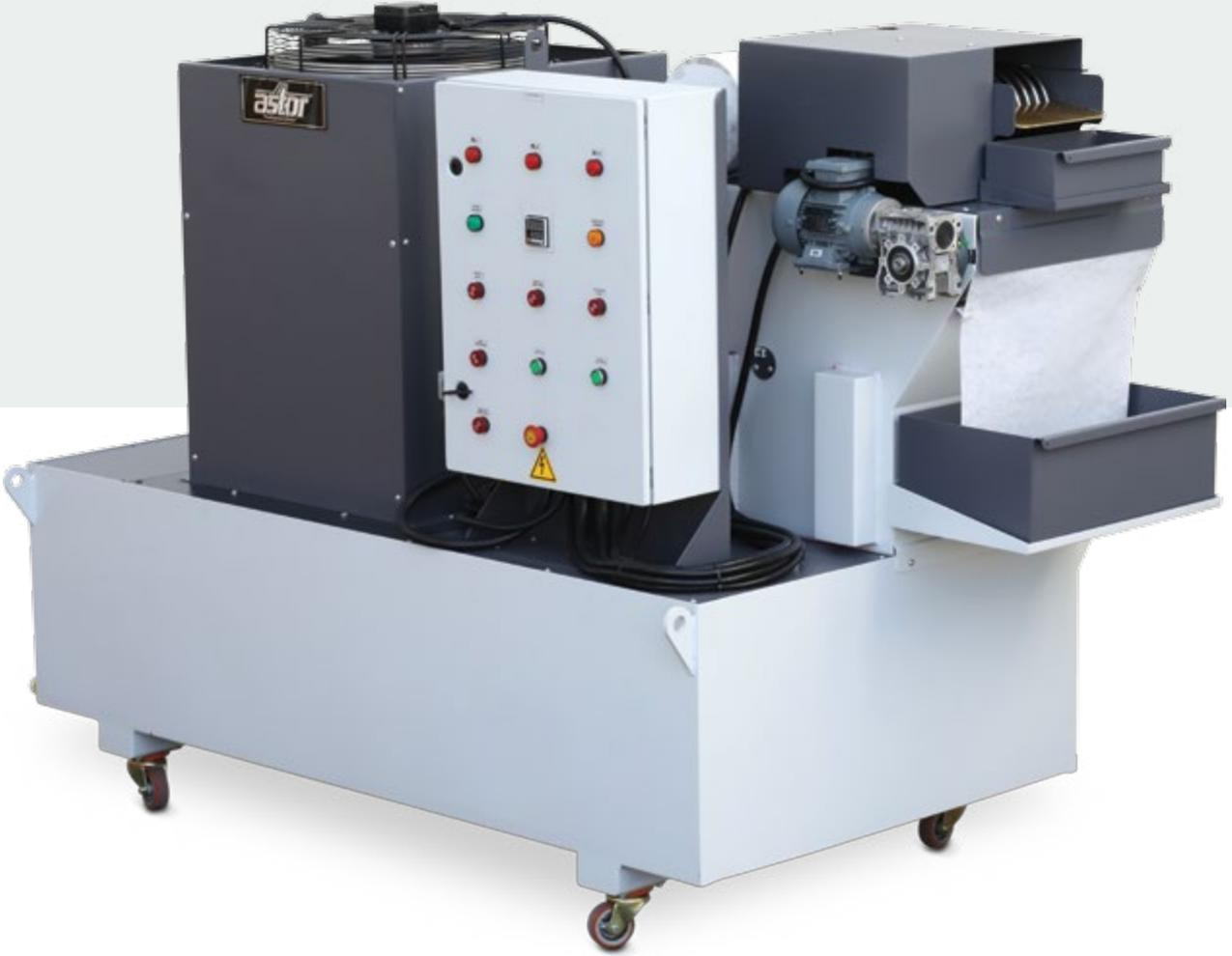
It is used for obtaining clean liquid up to 20 microns in machining centers, grinding and honing machines. It consists of magnetic separator, band filter and oil tank. Cooling unit and pump are added optionally.
