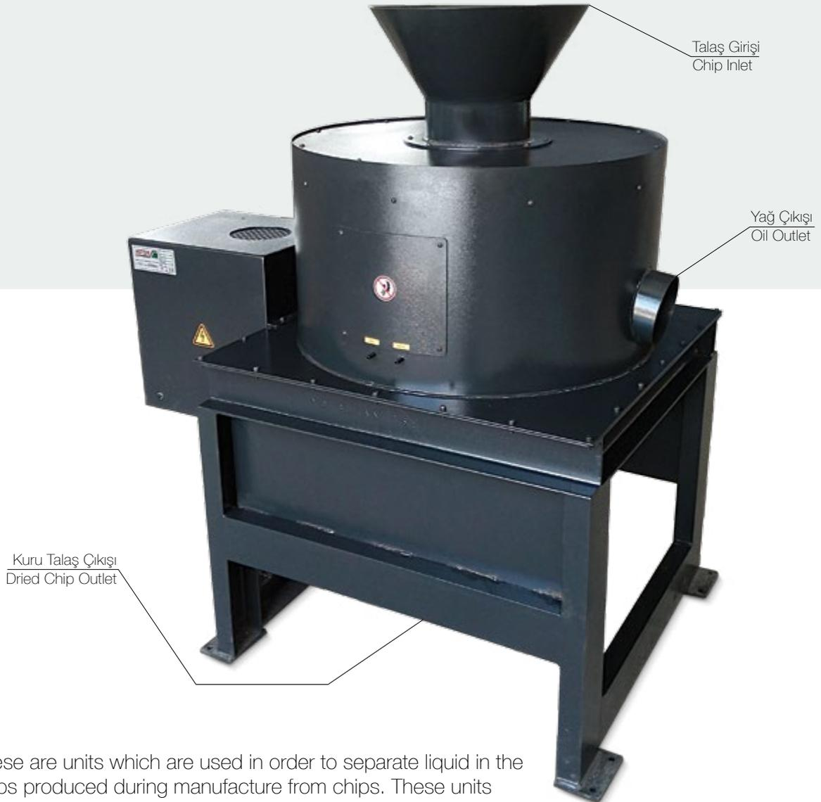
These are units which are used in order to separate liquid in the chips produced during manufacture from chips. These units reduce liquid waste occurring during manufacturing by recycling liquid disposed together with chips. Thus, waste liquid which his one of the most important factors that pollute the environment, is gained back. Chips are stored as dry for a long time in a healthy way and recycling is allowed. Chips are manufactured by considering centrifuged chip shape and sizes.
