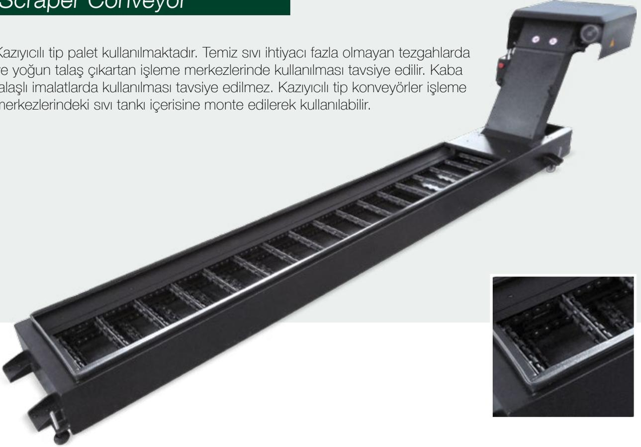
Scraper type pallet is used. It is recommended to be used in machines which don't need liquid a lot and processing centers which produce chips intensively. It is not recommended to be used in rough machining. Scraper type conveyors can be used by being mounted in liquid tank in teh machining centers.
