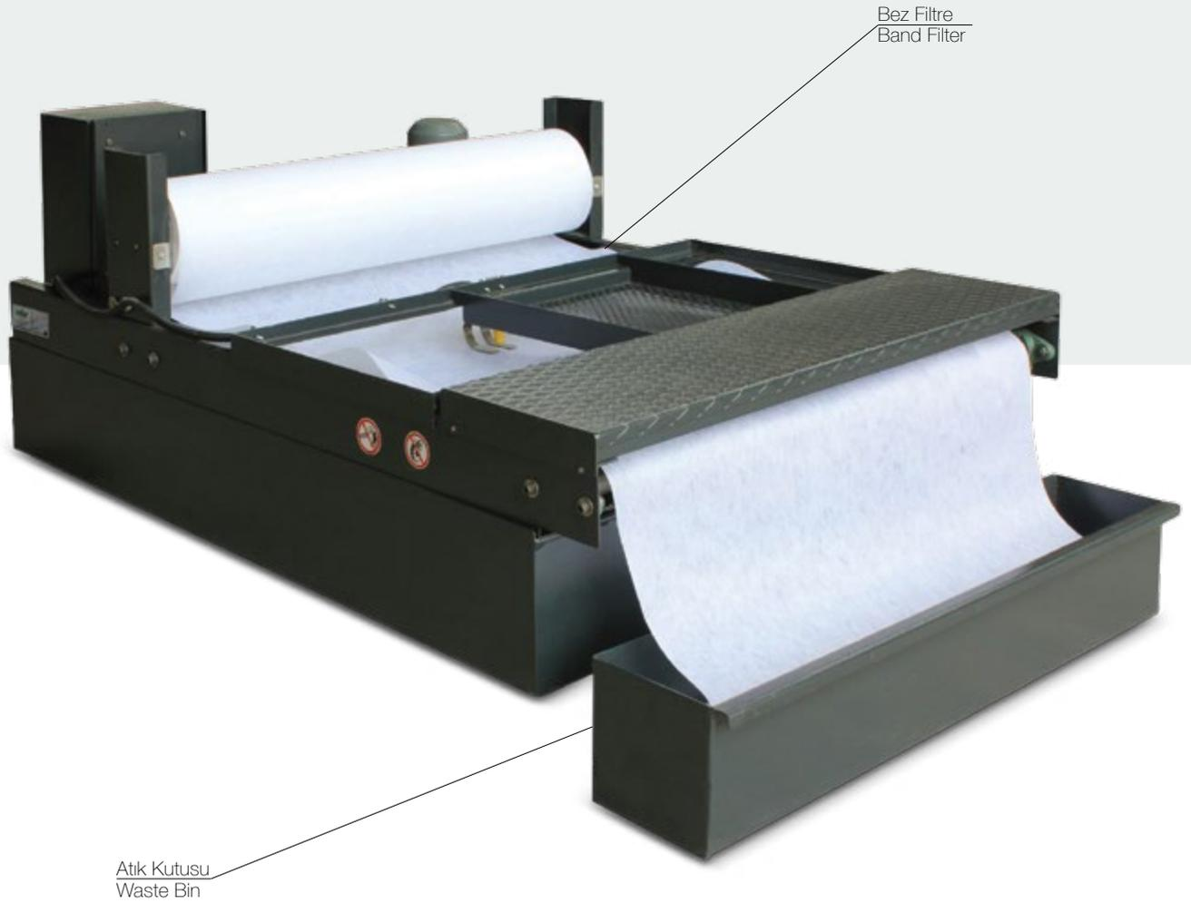
Foreign bodies in the liquid are filtered through band filter by filtration while dirty cooling liquid flows over unit by gravity. In this way, waste materials are collected with the help of band filter while clean water is being obtained.
